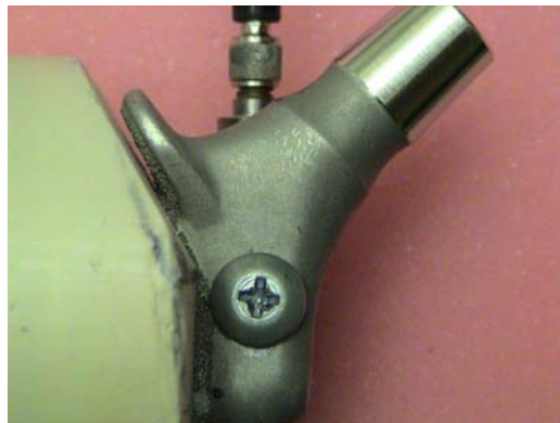
Figure 1. The femoral component inserted into the test bed with attached accelerometer.
