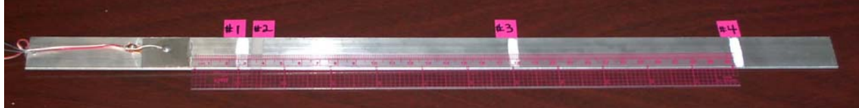
Figure 1: The 46 x 2.54 x 0.063 cm aluminum test structure shown with four levels of damage.
